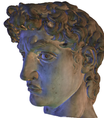
Figure 1: David head model rendered in Confetti as smoothly blended depth-sprites at a rate of 2M points/sec and 2 frames/sec.
