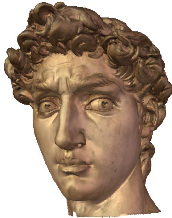
Figure 4.11: Splat based rendering example. The head of Michelangelo's David statue rendered using the Object Splat method by Pajarola et al.
