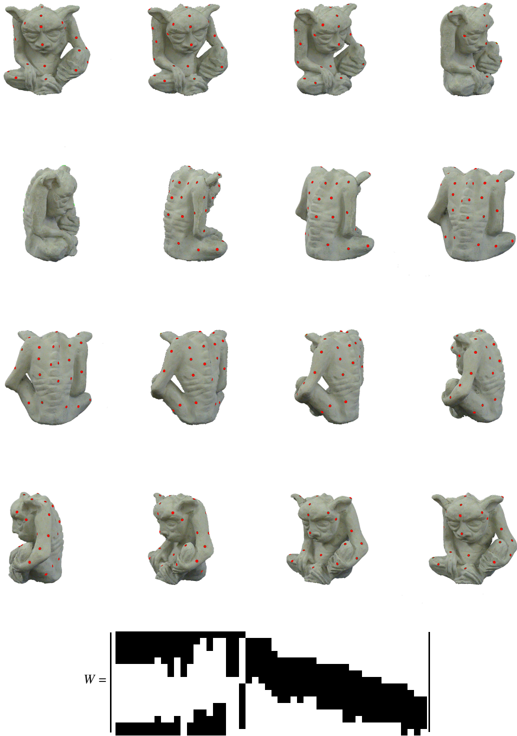
Figure 6.1: Input data for monster dataset. The 16 images used to reconstruct the monster dataset use a set of fiducials that can be seen as red dots on the surface of the object. At the bottom we see an image of the sparse measurement matrix for this dataset.
