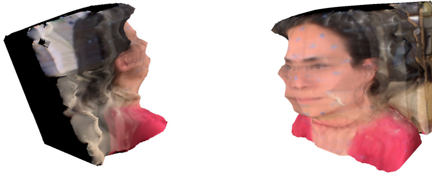
Figure 6.6: Example of space carving based reconstruction. The quality input images is low in contrast and color differences between foreground and background.
